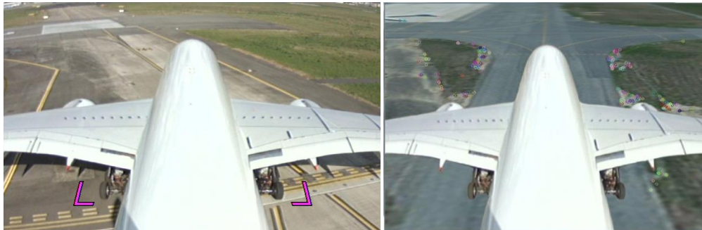
Figure 28. Image captured by a real camera mounted on the vertical stabilizer of an aircraft (left) and the image generated in Visuel superposing the aircraft body (right).
