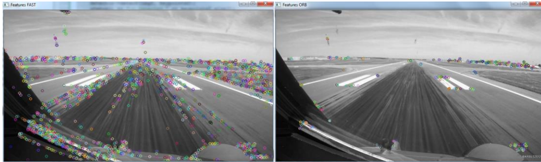
Figure 10. Examples of Feature Detectors included in OpenCV: FAST (left) and ORB (right).
