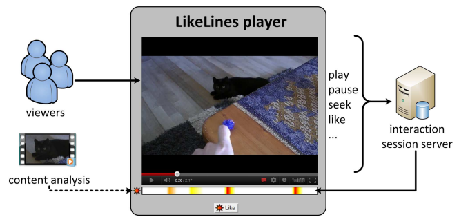
Figure 1: Users’ interactions (play, pause, etc.) with the LikeLines player are stored at a server and are aggregated into a heat map. Viewers can use this heat map to jump to a particular point in the video. Content analysis of the video can seed the heat map.
