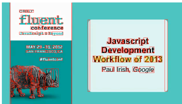
Figure 2. Connected components and their bounding boxes are used to draw highlighted rectangles over the main video canvas, giving users the illusion that they are selecting text from the video canvas.
